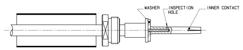
STEP 5- SLIDE CENTER CONTACT SUB-ASSEMBLY INTO THE OUTER BODY TIGHTEN THE CLAMP NUT: MAX TORQUE: 370N.Cm
